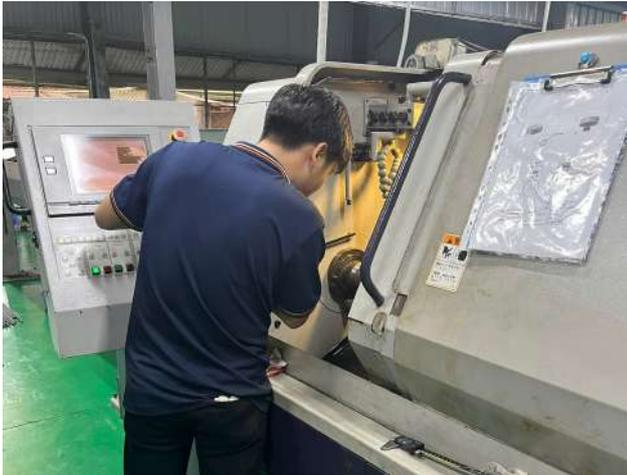
Our precision turning process uses cutting edge CNC lathes with live tooling. This means features like axial and radial holes, flats, grooves, and slots can be machined with accuracy.
